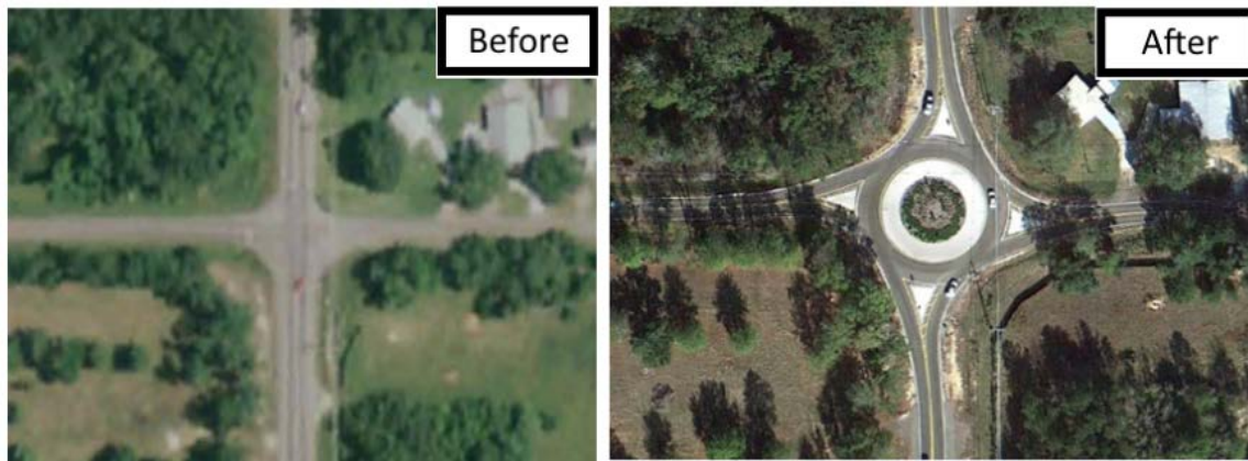
FIGURE 6 Before-and-after images of LA 3158 at Old Covington Hwy. roundabout.
